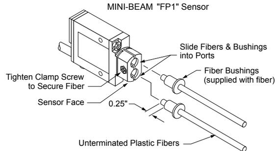
1. Prepare the sensor ends of the fibers (see [Cut the Plastic Fiber](#) on page 5).
