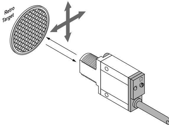
A highly reflective object may reflect enough light back to a retroreflective sensor to allow that object to slip through the beam, without being detected. This problem is called *proxing*, and the following methods may be used to correct it:
