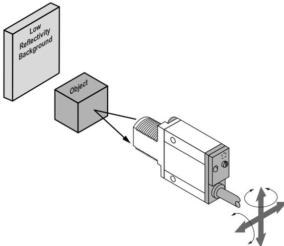
The sensing energy of a convergent mode sensor is concentrated at the specified focus point. Convergent mode sensors are less sensitive to background reflections, compared with diffuse mode sensors. However, if background reflections are a problem:
