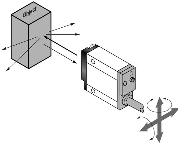
If the Alignment LED does not turn OFF when the object is removed from the beam, the sensor is probably detecting light reflected from some background object. To remedy this problem:
