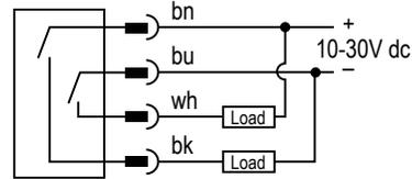
The output type for all models is Bipolar NPN/PNP; load 150 mA max., each output.
