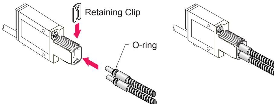
1. Install the O-ring (supplied with the fiber) on each fiber end, as shown in the drawing.
